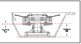
Distance from engine mounting surface to top of bearing
